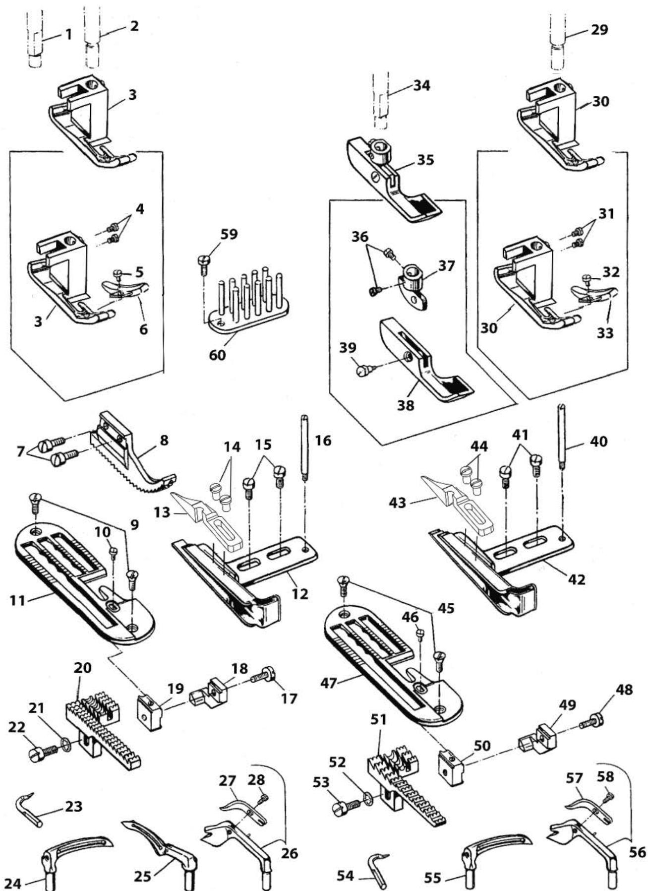
**SEWING PARTS FOR MACHINE STYLE 81200AC AND 81200AF**
