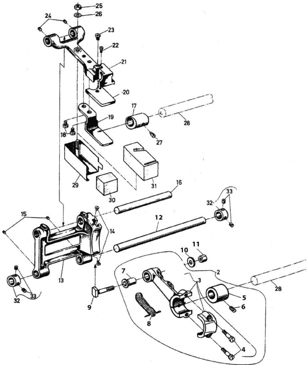
FEED LIFT AND FEED DRIVING PARTS FOR 81200EZ3254
