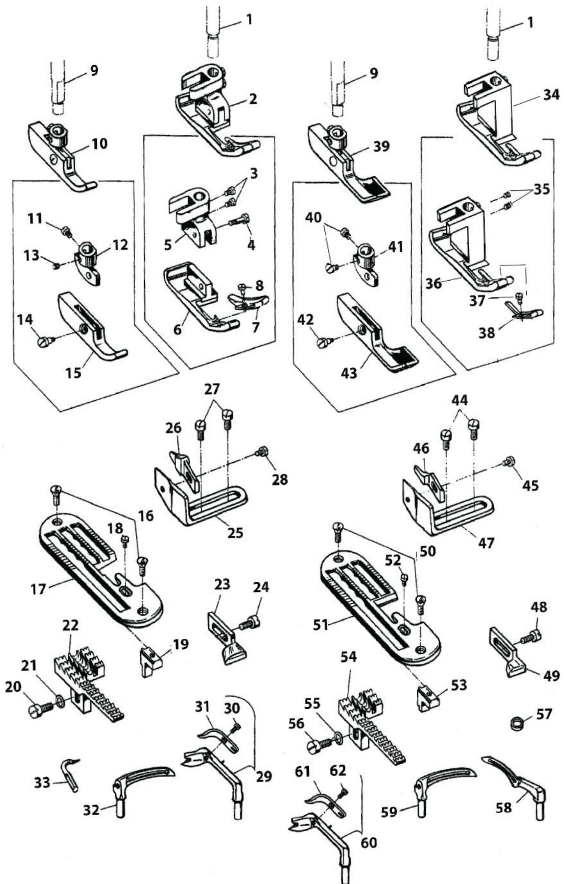
**SEWING PARTS FOR MACHINE STYLE 81200A**
